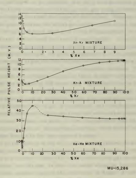
Fig. 11. Plots of relative pulse heights for xenon-krypton, krypton-argon, and xenon-helium mixtures.
